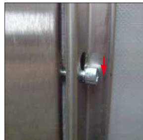
5 Put the hexagon socket screws of the stainless steel rail from the left through the key seats of the right rail and click them into place (downwards).
